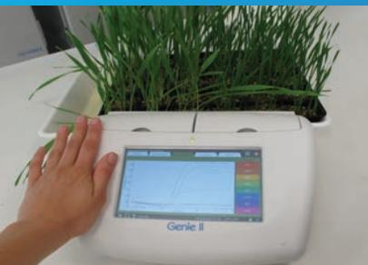
The LAMP machine is a small battery operated device that can be easily transported between fields
